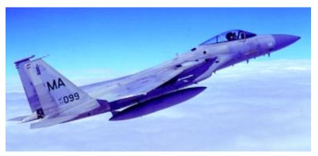
**Weight:** empty 45,000 lb, gross 81,000 lb. **Ceiling:** 50,000 ft. Performance: max level speed at altitude Mach 2.5, ferry range with CFTs 3,000 miles.
